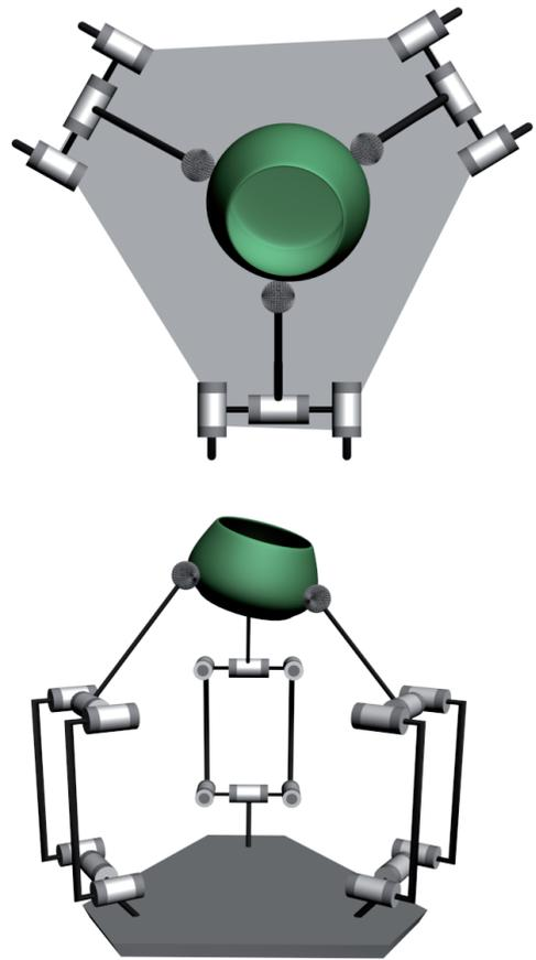
Fig. 3. Manipulable grasp with 6 degrees of connectivity.
