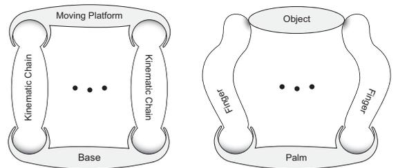
Fig. 1. Topologies of a parallel robot and a palm-fingers-object system.
