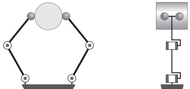
Fig. 2. Planar manipulable grasp with 3 degrees of connectivity.
